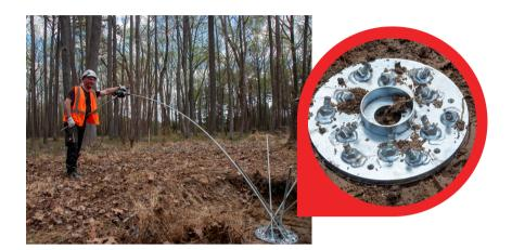
Based on the root system of a tree, the Spinnanker system is engineered to deliver superior holding strength in almost any soil type.
